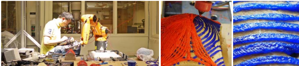
Figure 7: Fabrication shop workspace for KUKA operation and filament extrusion
