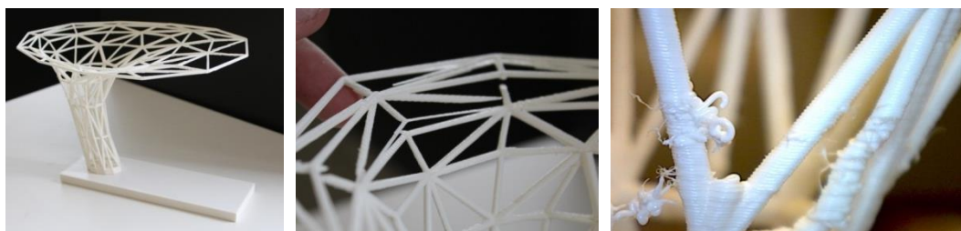
Figure 8: Three-dimensional grid shell model made in ABS with FDM with print-orientation issues.
