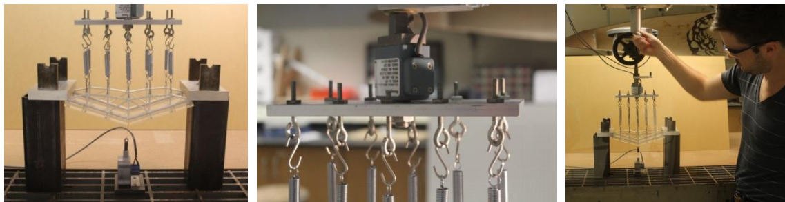
Figure 5: Load test setup, showing two parallel truss models, acrylic bracing plates, spring load-spreading system, and aluminum plates for loading and supports.
