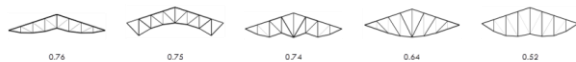
Figure 11. Robert Maillart's 1924 design for a shed roof in Chiasso, compared with designs discovered using the computational approach presented in this paper.
