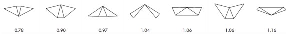
Figure 8. A closer view of several candidate designs created by the population generator and presented to the user, with scores normalized by a base design's score shown underneath each.
