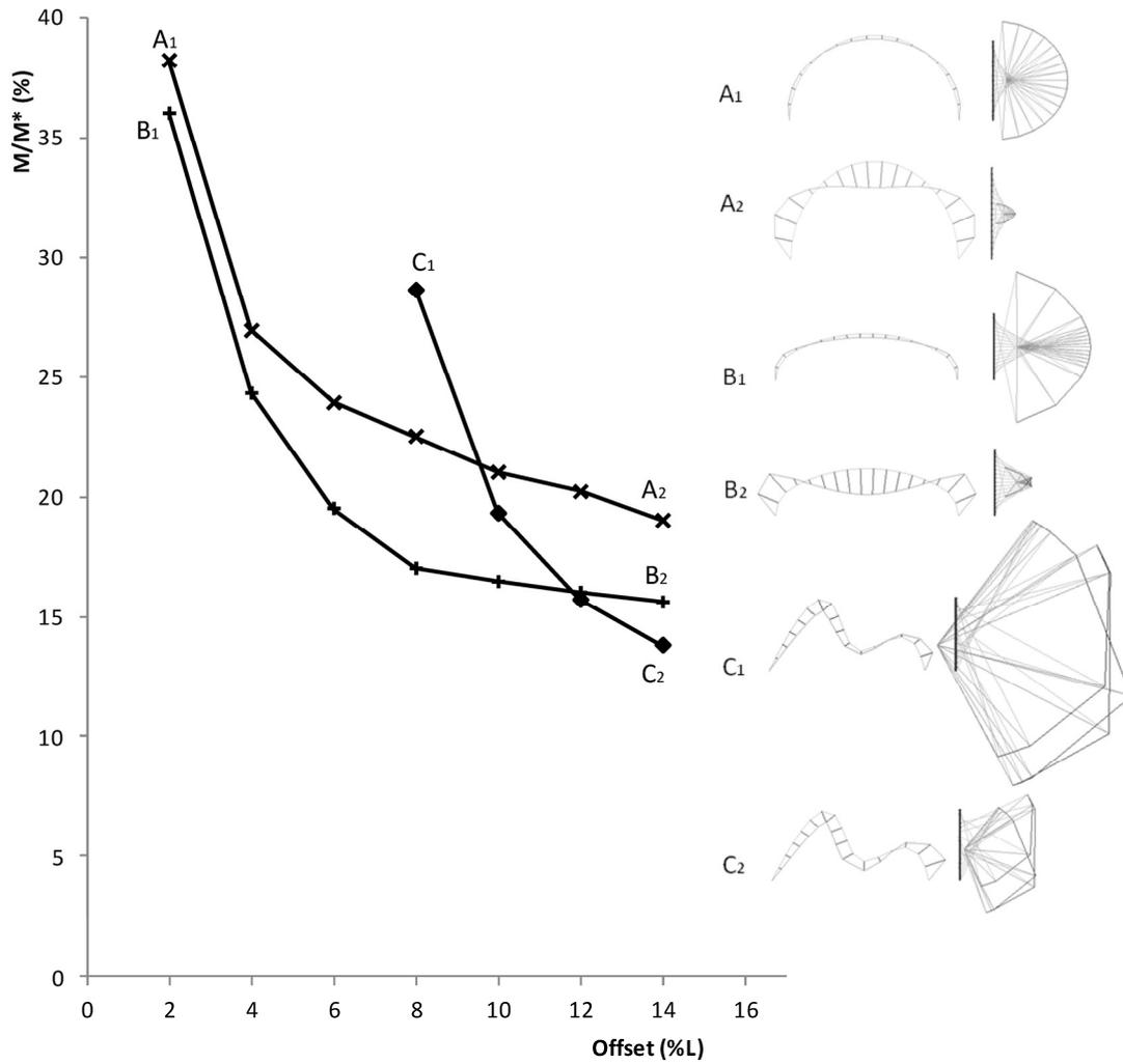
Figure 5. Comparison between bending and post-tensioned solution for a three-pointed arch, a semi-circular arch and a free-form curve with different offsets.
