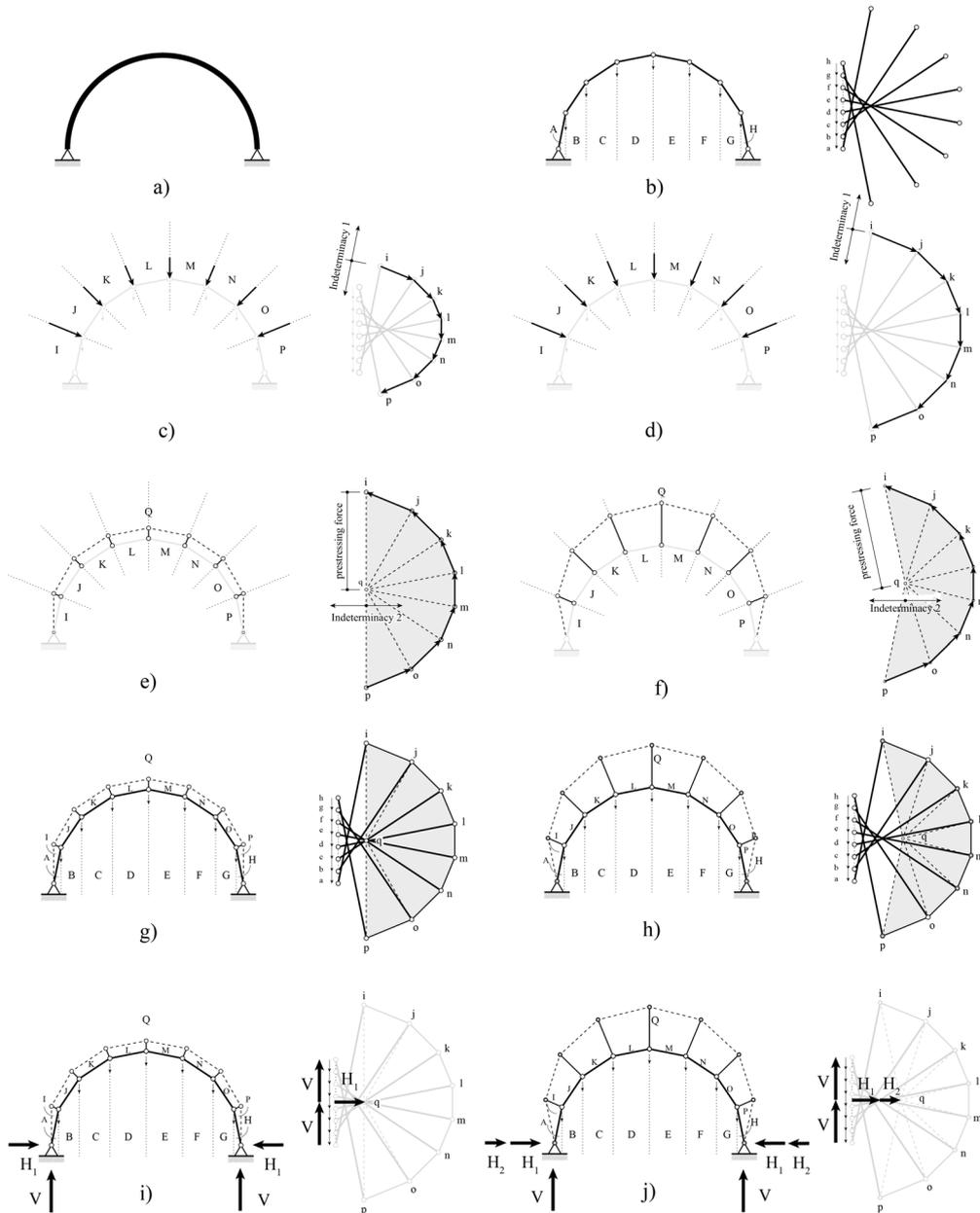
Figure 2. Graphical construction of the external post-tensioning system.
