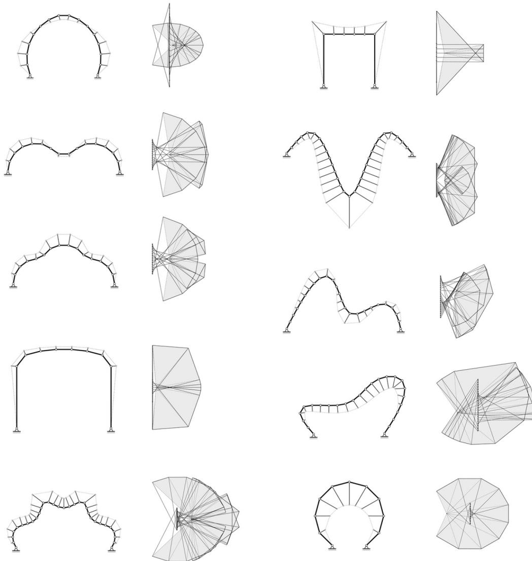
Figure 4. Examples of resulting post-tensioned forms for arbitrary geometries.
