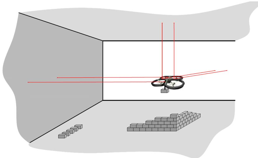
Figure 5: Positioning system based on 3 pairs of lasers
