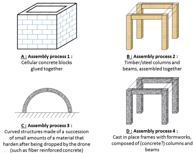
Figure 4: Examples of drone compatible assembly processes (DCAP)
