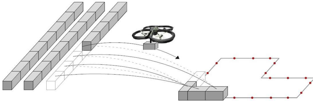
Figure 13: Flying routes that the drone has to follow between the storage location and the dropping points
