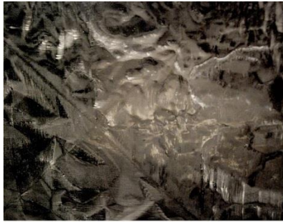
Figure 19: Looping texture produces more dispersed light and opacity
