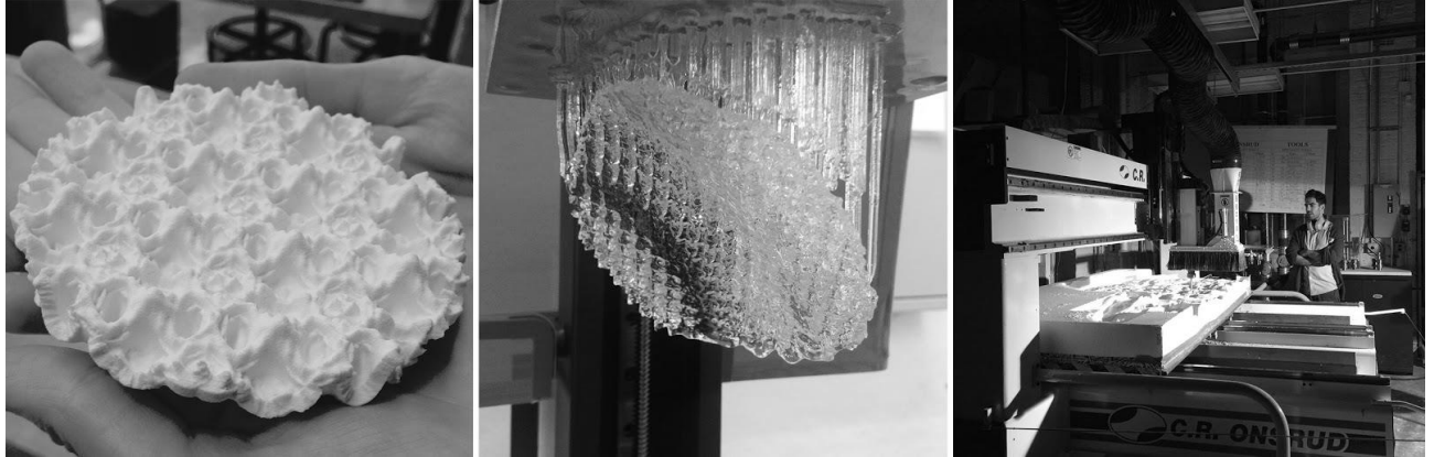
Figure 10: a) Additive manufacturing: powder printed models were brittle and did not have useful mechanical properties b) Additive manufacturing Optical qualities - resin stereo lithography on a Form-1 3D printer, c) CNC milling
