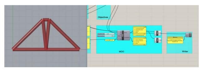
If the designer would like to consider only a single design from the sampled design space, this can be achieved using **Sift**. Although resetting the variable bounds is fairly trivial for this problem, it is more labor-intensive for parametric problems with more variables.
