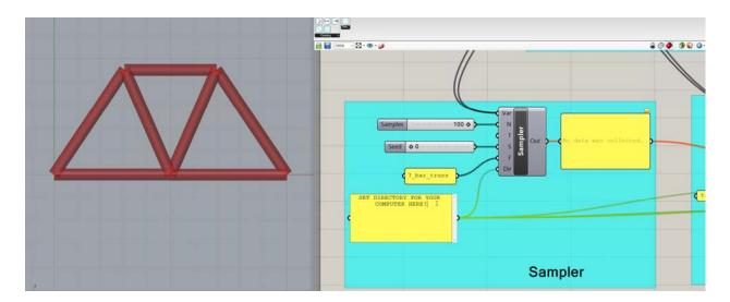
Once the Directory is set, the rest of the components will become functional. To take a representative sample of all potential truss options, doubleclick the **Sampler** component. This creates a Design Map of potential truss variable settings:
