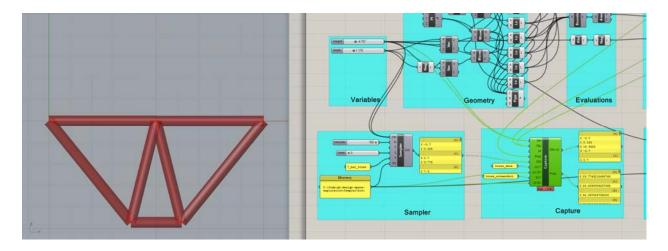
The shot above shows Capture outputting both the new Design Map + Objectives, as well as a corresponding list of design properties.
