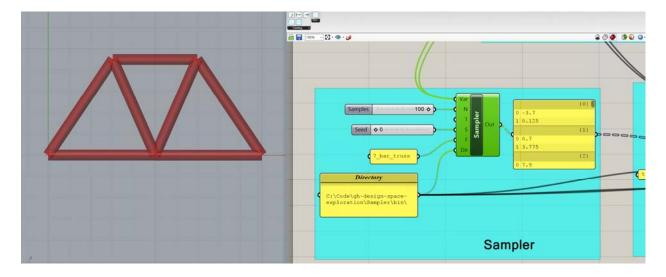
Alternatively, the **Reader** component could be used to read in a Design Map previously saved in a Directory.
