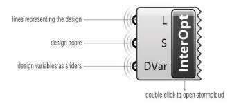
Connect the input parameters of the component to the lines representing the design geometry (data must be flattened), the design performance score (as a number), and the design variables as sliders. The exploration will be performed around the initial value of the sliders. Hence, the user may want to reset the sliders to their middle values.
