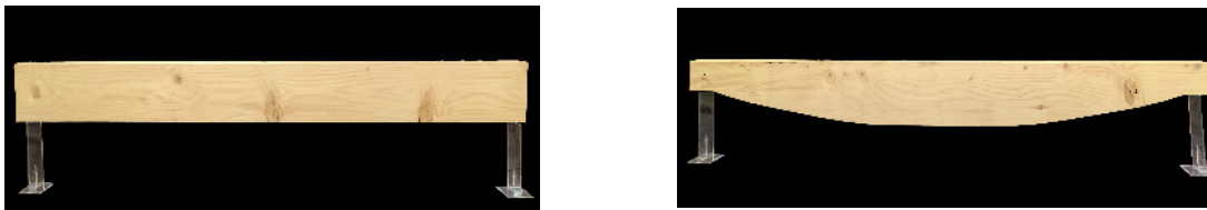
Figure 6: Left: initial beam. Right: timber beam shaped for height
