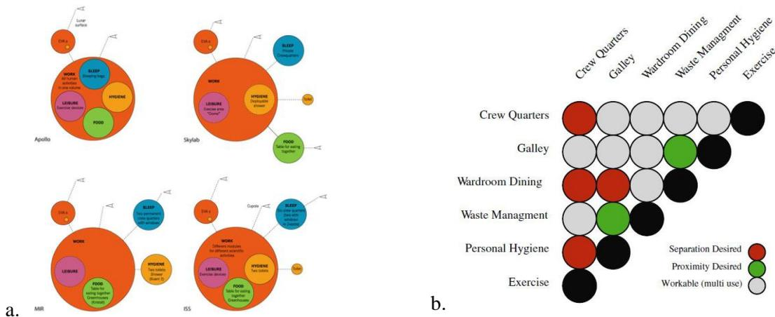
Figure 4: a. Bubble diagram [11], showing the preliminary zoning of the Lunar Lander, Skylab Station, Mir Station, and the International Space Station; b. Adjacency matrix for the collocation of functional zones.
