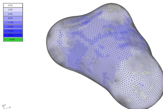
Figure 9: Tensile stress distribution inside the inflatable structure.
