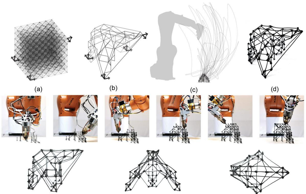
Figure 3: *3D cantilever* case study, with (a-b) topology optimization input and result, (c) robot trajectories, and (d) final extruded result
