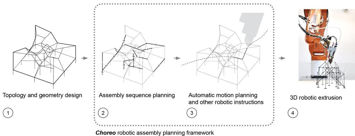
Figure 2: Overview of the robotic extrusion workflow including the automated planning system
