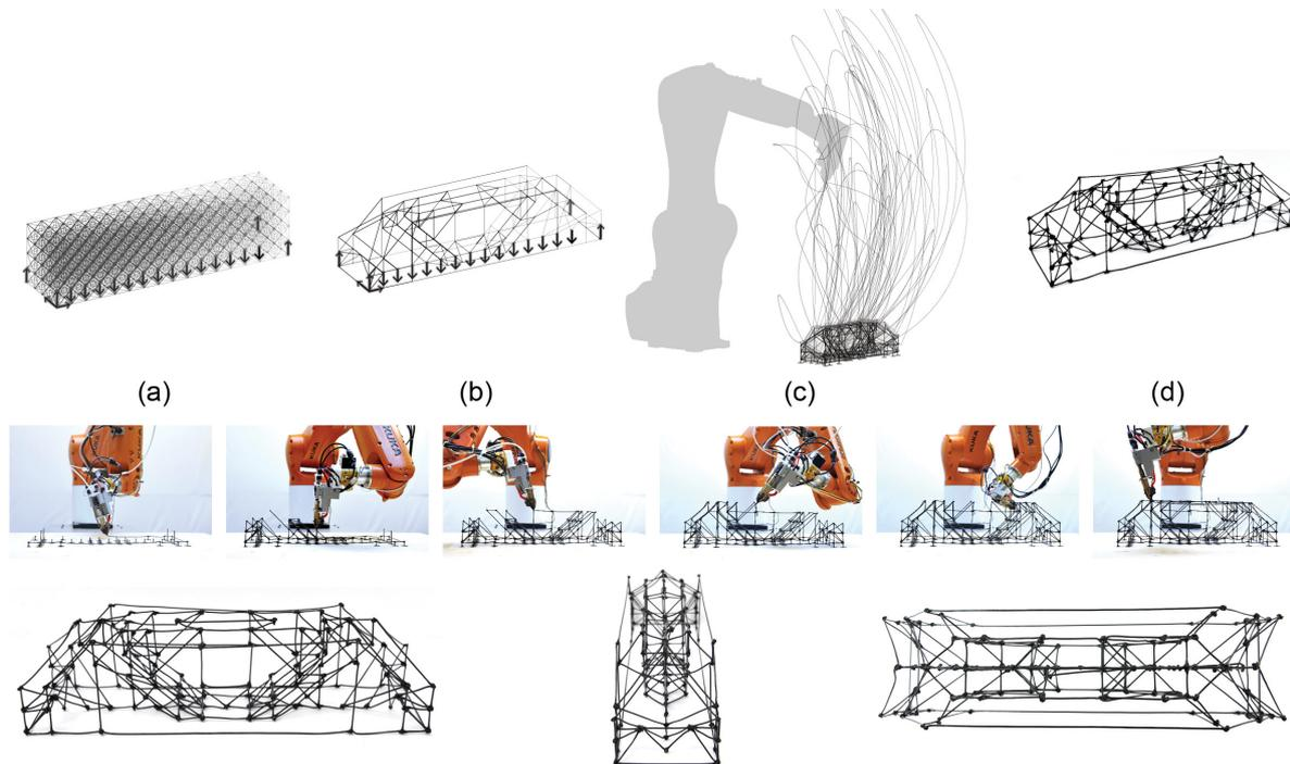
Figure 4: Simply supported beam case study, with (a-b) topology optimization input and result, (c) robot trajectories, and (d) final extruded result
