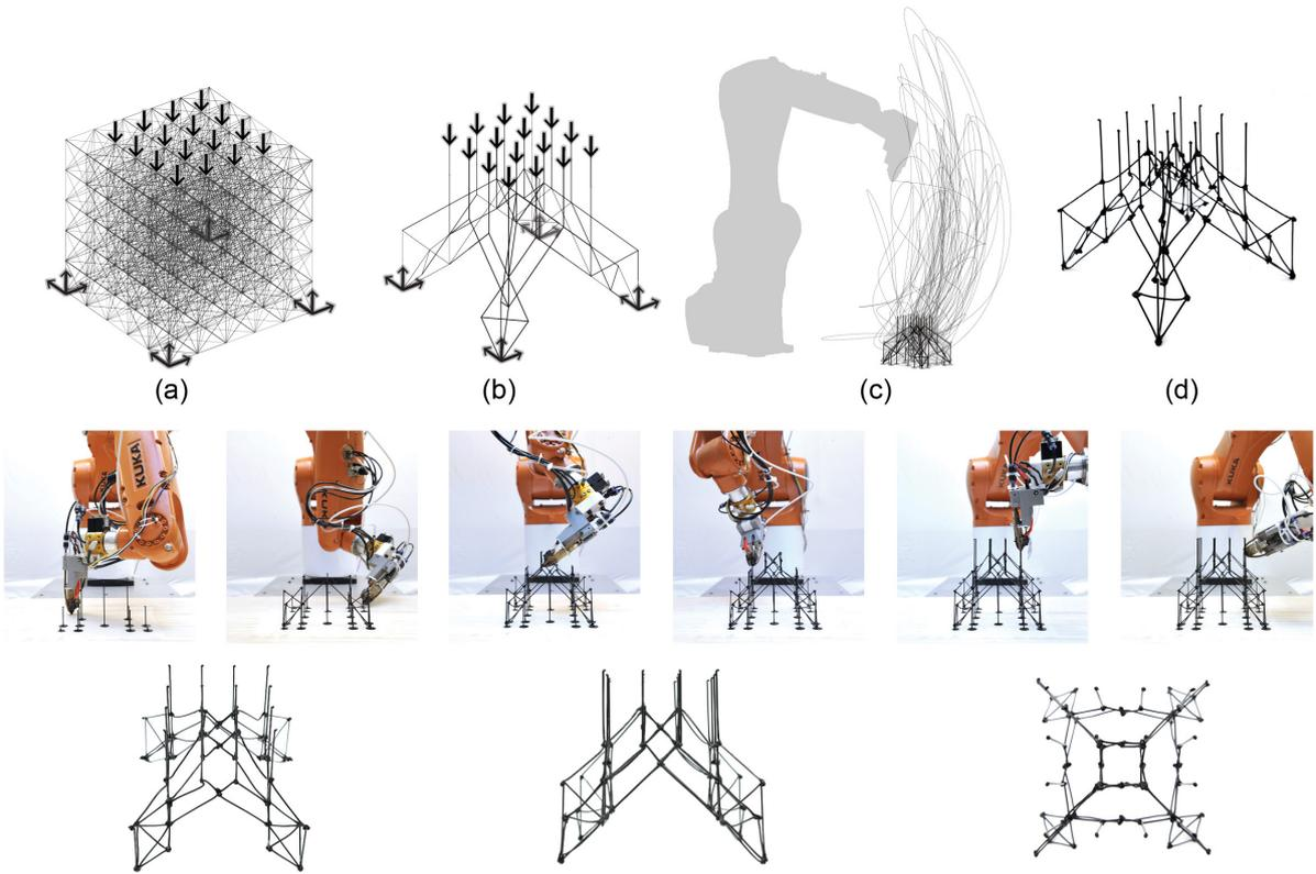
Figure 2: *Vault* case study, with (a-b) topology optimization input and result, (c) robot trajectories, and (d) final extruded result
