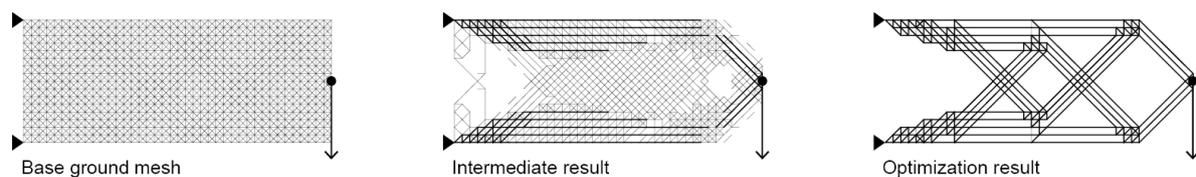
Figure 1: topology optimization process for a 2D cantilever setup
